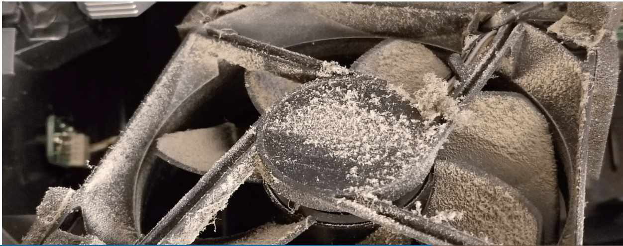
Figure 5- Dust inside a high-powered laser projector can shorten its life if it is not sealed and IP5X certified.
